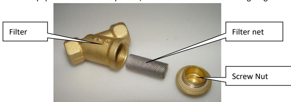
After removed the nuts, remove the filter net, clean the filter impurities by clear water. After leaning re-install it. Cleaning of solenoid valve
