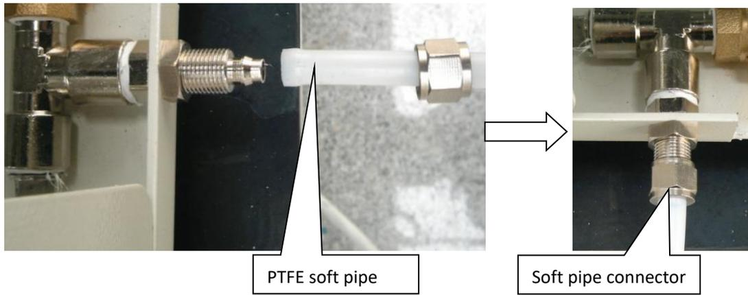
When discharging the residual water in steam generator, please operate in accordance with the following steps:
