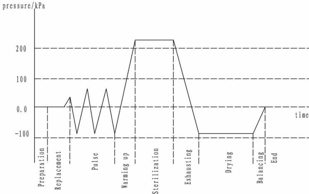
Instruction: When the product is not equipped with the vacuum function, the process is the positive pressure pulse
