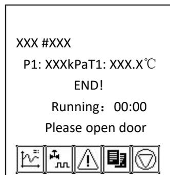
The interface displays the name of each phase, chamber temperature and pressure value. A sterilizing cycle includes the following phases:
