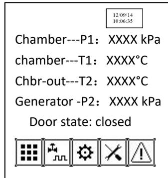
Chamber-P1: Indicates the chamber pressure
