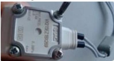
Remove the 4 screws of the solenoid valve.
