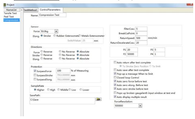
Sensors: the choice of force and displacement sensors
