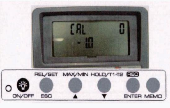
5. Set FLUKE AM-011 output is 57mV, than press [Max/Man] Key, the [57] will blinking in LCD of upper right corner.
