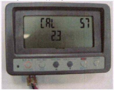
6. The [57] will stop to blinking in LCD of upper right corner after few ten second. The CAL is completed, than the meter will move to Measure Mode and CH1 will display E3 and red LED will blinking and ALM is on.
