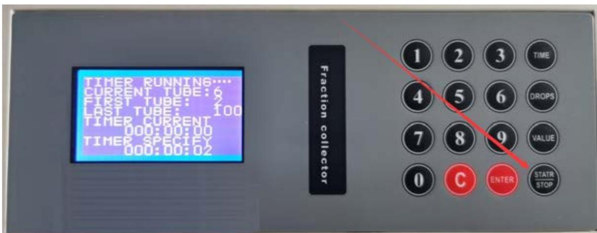
After running to the end of timing collection of tube 100, the instrument will alarm automatically,
