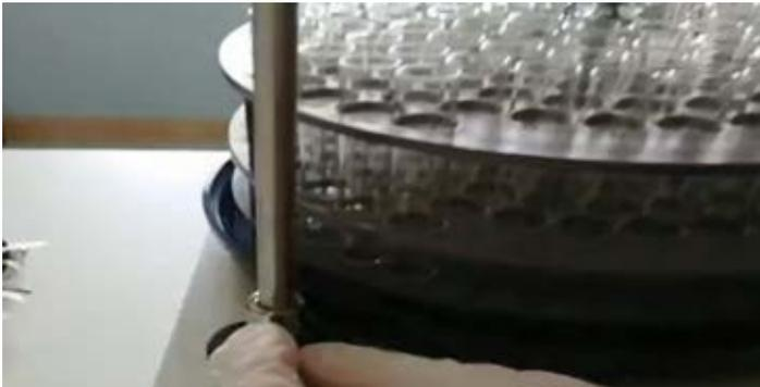
4. Fix the "safety valve" on the upper part of the "vertical bar"
