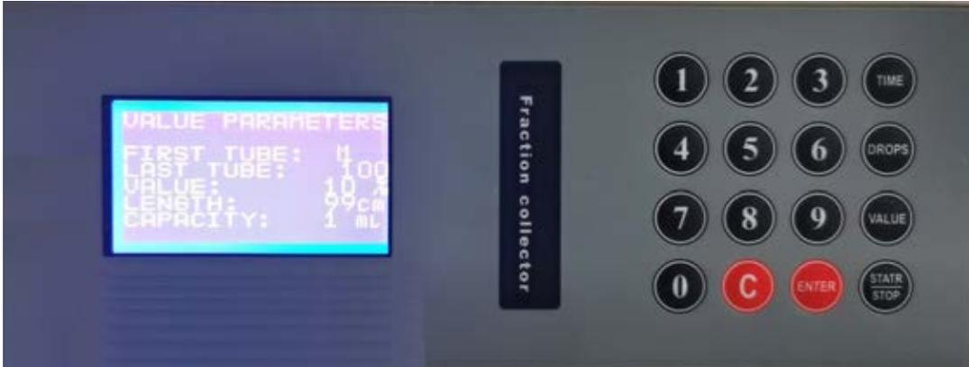
The "first tube" is set to "3" and press "confirm" button;
