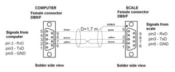
Scale - computer cable diagram for plastic casing
