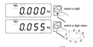
• The inscribed value confirm by pressing , the program will automatically go to the higher threshold of weighing (**Max**):
