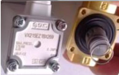
Lift the valve head vertically. Keep the spring stays on it.
