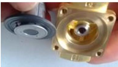
Take out the movable core and seal ring to view the sealing surface of the valve.
